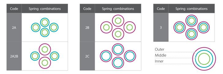
Sizing a spring return actuator requires that the torque output at the start and end of both the spring and air drive strokes is greater than the valve torque at that position.
